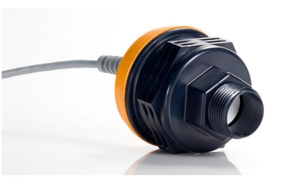
Ultrasonic sensors work by transmitting energy in the form of ultrasonic waves to a target object, which reflects the waves back to the sensing head. Ultrasonic sensors are largely used in measuring distances based on the time it takes for the wave transmission and reception to be completed.
